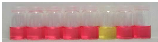
Figure 2. Colour variation observed in acetonitrile solutions of L^2 ( [L^2] = 1.1 \times 10^{-4} \text{ mol dm}^{-3} ) in the presence of 1 equiv of certain metal cations. From left to right: L , \text{Ag}^+ , \text{Cd}^{2+} , \text{Cu}^{2+} , \text{Fe}^{3+} , \text{Hg}^{2+} , \text{Pb}^{2+} , \text{Zn}^{2+} .
